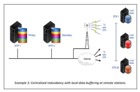
This application uses a reportby-exception scheme to report data and alarms from 26 remote sites and record it to a pair of collocated historical databases located in the central control room. The Historian directs data storage, synchronization services and bi-directional data backfill between the databases.
