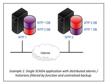
WTP1 includes a historical database, which is used for primary storage of local data and backup storage of data from WTP2. Conversely, WTP2 includes a 2nd historical database, which is used for primary storage of local data and backup storage of data from WTP2.
