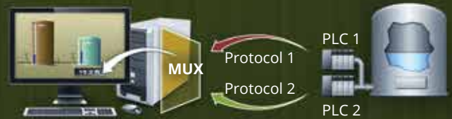
Failover to redundant networks or devices.
