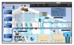
Pump Station Display Created by Star Controls within VTScada
