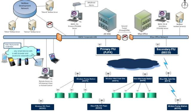
Blue Hills Distribution SCADA System Network Diagram
