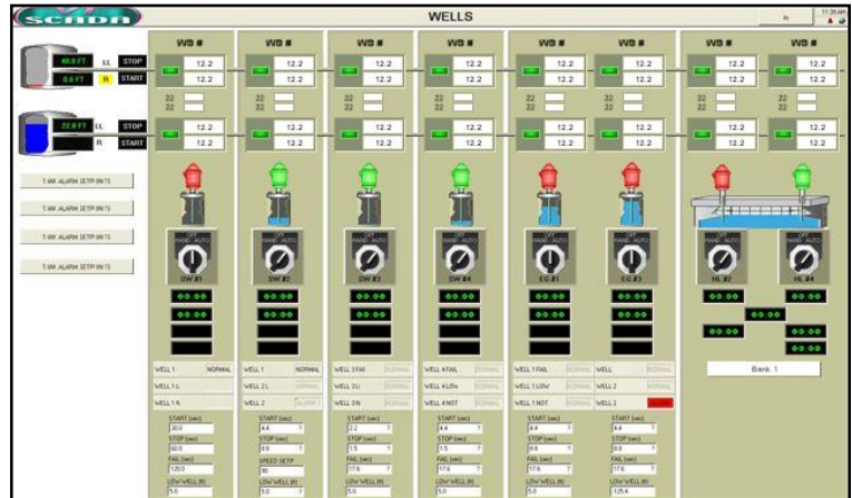
A well overview display created with VTScada HMI software.
